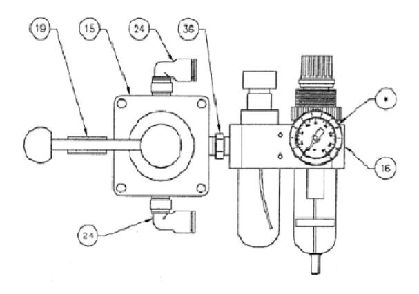
View shown is for D-10P, D-20P, D-20SP, and DK51. Swivel Hand Valve (#15) 180° and mount the gauge (\*) on the opposite side for D-50SP and D-100SP assembly. Tube fitting (#24) is turned straight out on D-10P assembly
