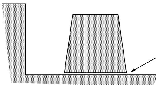
If mortar gets between the insert and the mould surface, demoulding will be difficult
