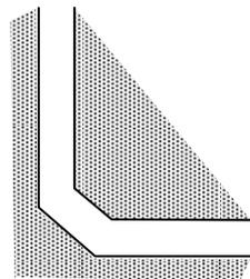
Radius or chamfer corners wherever possible
